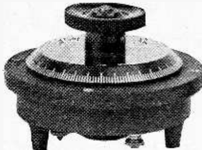
The compact variometer recently produced by the Dubilier Condenser Company.
